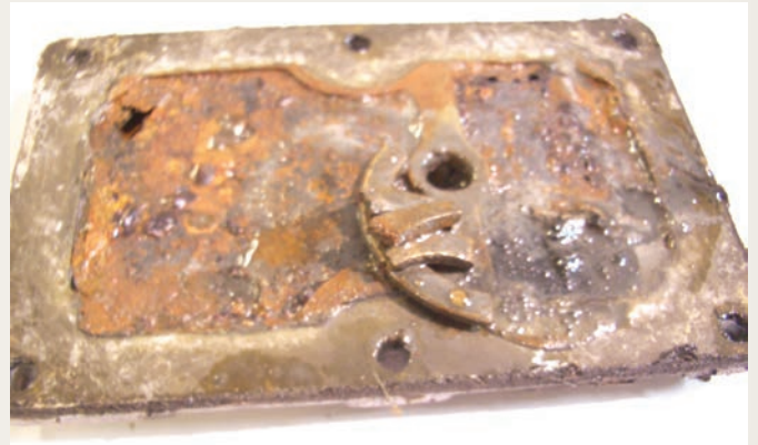
This LH-type Overdrive will need more than an oil change!
