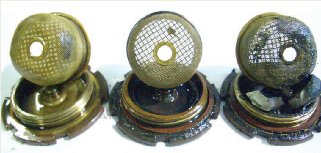
A-type filter and plug: The Good, Bad & Ugly.
