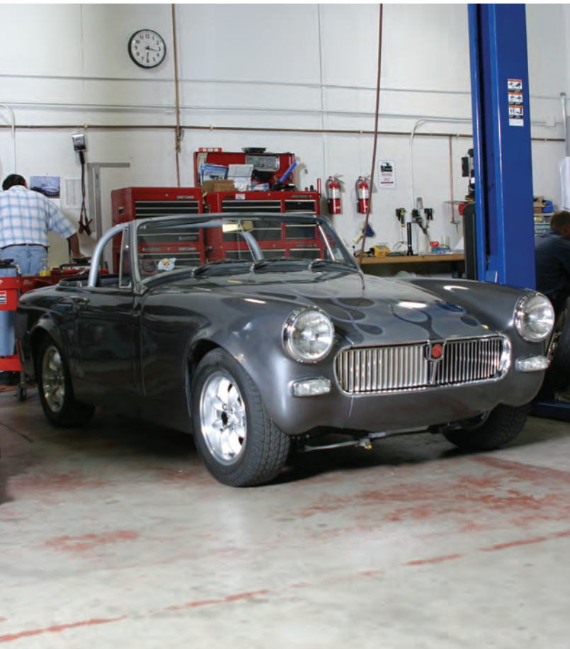
Moss Motors co-owner, Robert Goldman, says his MG Midget is the car he should have had when he was 18. Named The Flaming Cockroach, he says the car is a mongrel, with a '73 tub, early grille and lights, and a variety of parts from the bin. It boasts a Moss supercharger, Mini Cooper S cam, aluminum flywheel, aluminum cylinder head with port work by Sean Brown at Flow Speed, a long center branch header, and billet four-pot brake calipers by Kent Auto Developments.
