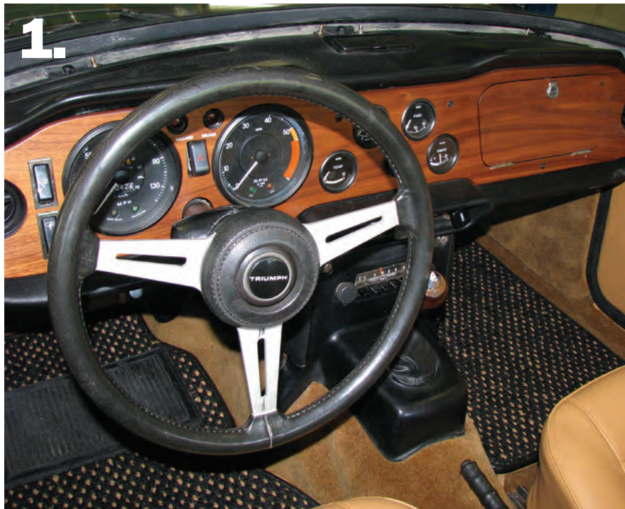
1. The stock steering wheel looked pretty good, but it wasn't a good fit for our early Triumph TR6. It also puts your fingers too close to the switch gear.
