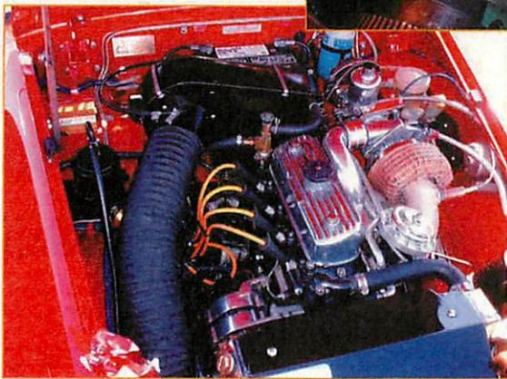
Wherever advantageous, I adapt components from other British models in the style of BMC/Leyland engineers. I changed over to the large diameter Austin Mini water pump pulley and the bigger MGB alternator pulley to slow these belt driven units down.
