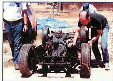
The engine and transmission are installed.
