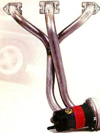
✓ Install header, upgrade exhaust system.
