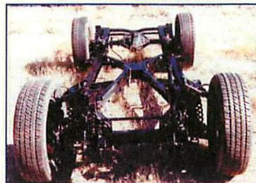
Stripped frame and suspension ready for engine.
