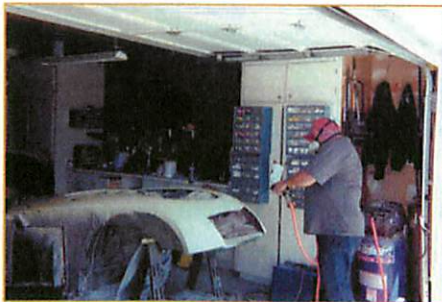
Bryan Lacasse sprays a primer coat on the MGA's "body."
