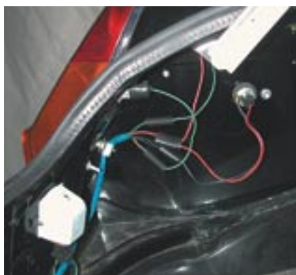
The Moss Third Brake Light kit includes a Hella lamp, a pigtail wiring harness, 4-way connectors, a magnetic base, and an adhesive-backed gasket for the magnet.
