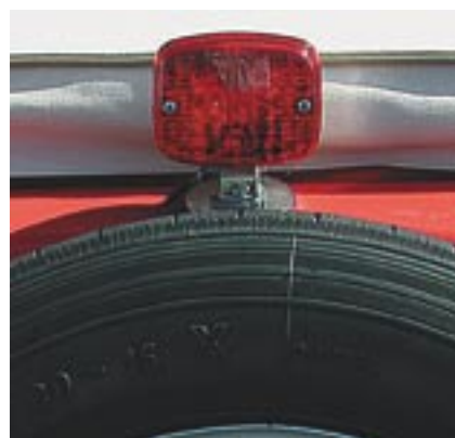
The Moss Third Brake Light kit includes a Hella lamp, a pigtail wiring harness, 4-way connectors, a magnetic base, and an adhesive-backed gasket for the magnet.
