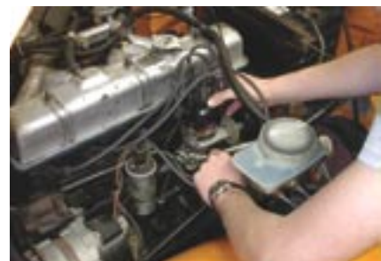
1. The first step is to remove the distributor cap and push it out of the way. Do not remove the spark plug wires.
