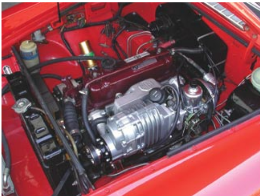
It's hard to argue with the wow factor when you open the hood and reveal the Moss supercharger system. Nice details such as the MG logo cast into the manifold and the new SU carb make the supercharger system appear period-correct.
