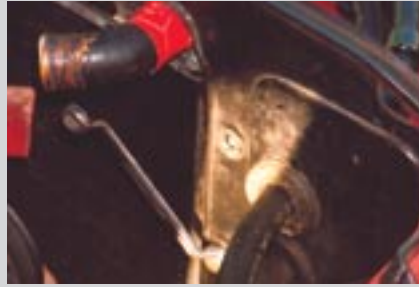
1. Release the bolts that secure the radiator to the radiator support.
