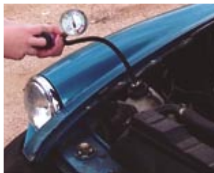
The pressure tester replaces the cap, either on the radiator itself or on the expansion tank if so equipped.
