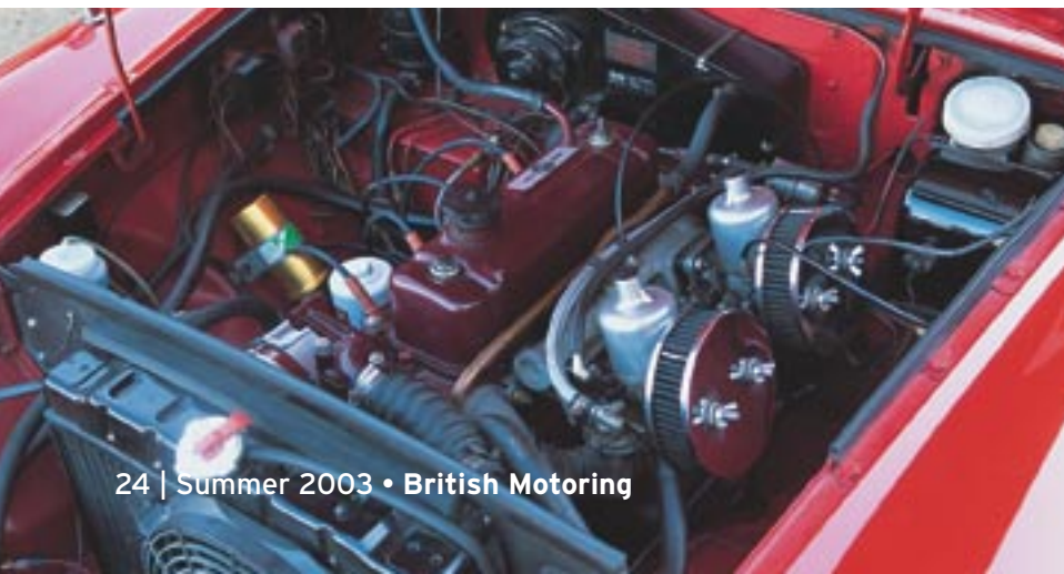
When in doubt, bore it out: Masquerading as a 1.8, Tim's bored-and-stroked 2.1 makes about 100 hp at the rear wheels. A K&N oil filter is one of the few visible performance parts
