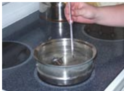
Use a pan of heated water and a thermometer to check the thermostat. The spring should begin to retract at the thermostat's rated temperature.
