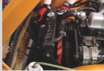
4. Check clearances, then mount the fan in the desired location on the radiator or AC condenser. Carefully push the four mounting-rod assemblies through the fan's brackets and cooling fins, securing with a locking button on the other side.
