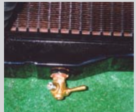
5. Replace the hoses as necessary before reinstalling the new or rebuilt radiator. Early MGB brass drain plugs can be retrofitted with a petcock to facilitate draining. Reinstall the radiator by reversing the disassembly process.
