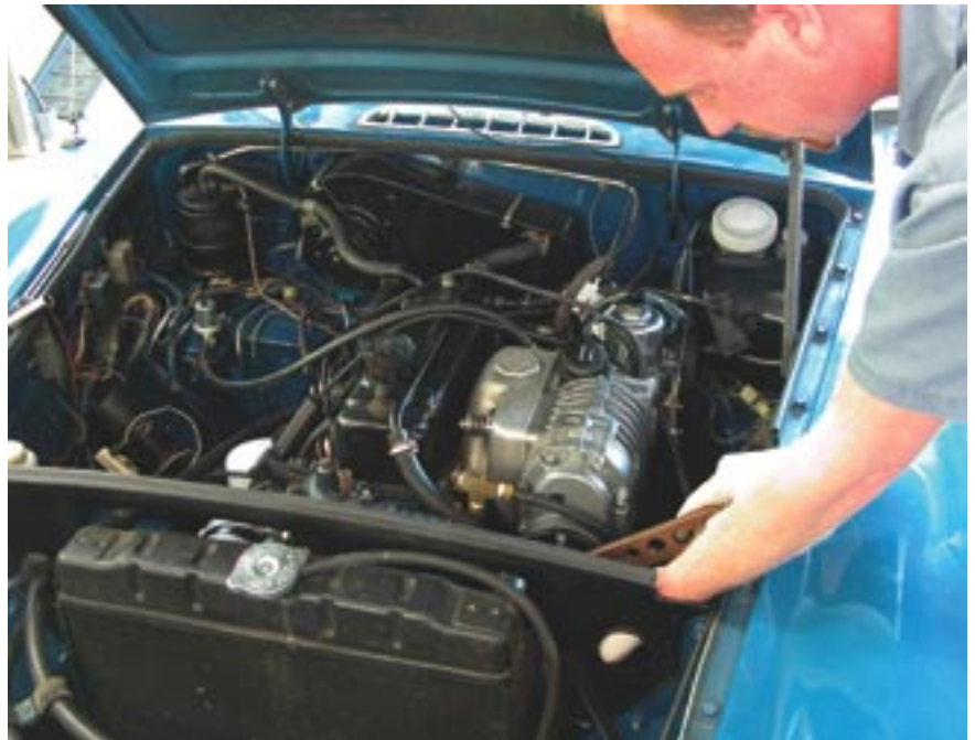
Different pulley sizes were tested to vary system boost pressure. The engineering challenge is to find the ideal combination of boost-induced power without compromising reliability.
