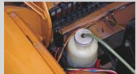
8. The relay and fuse (not visible) are securely mounted, both ground wires are double-checked for secure contact, wires are secured with nylon ties, and the fan is tested.
