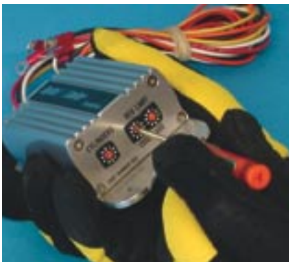
Rotary switches on the side of the rev limiter are for number of engine cylinders and rpm cut-out level. The customer can easily set the rpm limit with 100 rpm accuracy by turning the switch dials. Setting all switches to 0 makes the unit non-operational.
