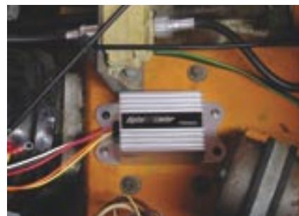
Optimal mounting location for the rev limiter is a reasonably flat surface that's away from direct heat, vibration, and moisture.
