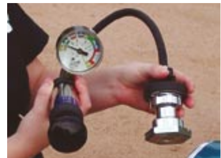
Most pressure testers have an adapter to check cap function. If the cap won't holding its rated pressure or won't release above that rating, replace it.
