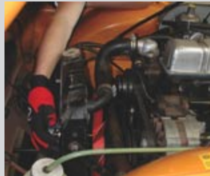
5. Locate the temperature-control rod the specified distance below the water neck and carefully insert it through the fins. Remove the rod, snap off excess length, screw on the snap switch, reinsert the rod, and secure with the foam pad and locking clip.
