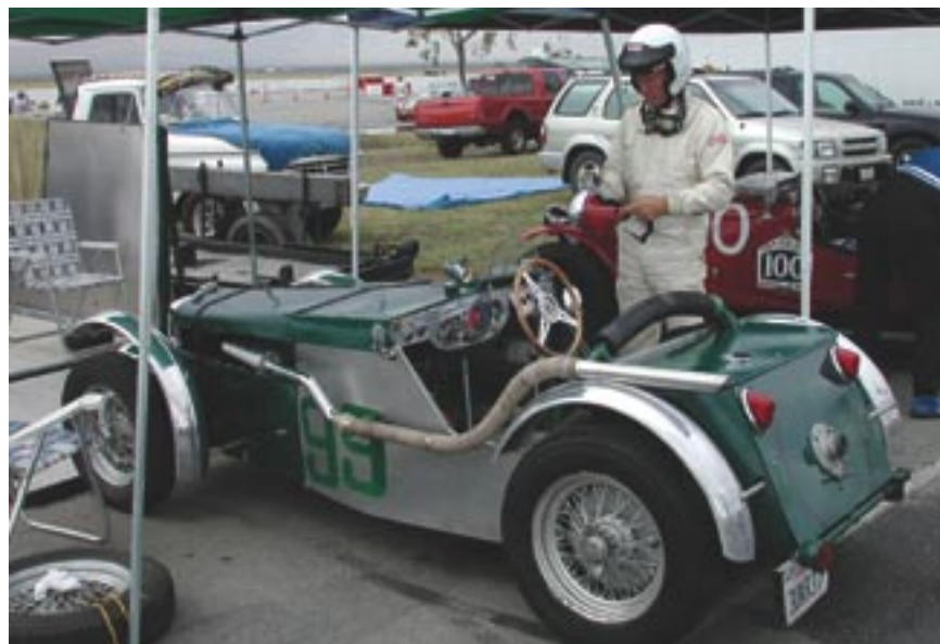
From any angle, this MG N Special looks "right." Rudge wire wheels were cut down from 18 to 16 inches. Brakes have been converted to hydraulics in front but retain cable-operated rears. A few parts were carried over by MG from the N-Type to the TA-B-C, notably the rear axleshafts and electrical parts.
