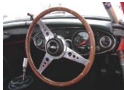
The nice thing about vintage race cars is that their interiors closely resemble real production cars. Shifting with your left hand in this right-hand-drive Healey gets interesting when you start using overdrive in third and fourth gears. The car has a production BJ8 gearbox and a straight-cut-gear Tulip competition gearbox that will go back in with the race engine. You can see a hint of the custom-built roll cage. Other features are the Connelly leather interior and Denis Welch racing seat.
