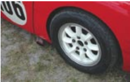
#106 came with two sets of Panasport Lite racing wheels. When it was prepared for the DMH race at Le Mans it was converted to FIA spec with wire wheels. Four-wheel-disc brakes and a limited-slip differential are used for Vintage Racing.
