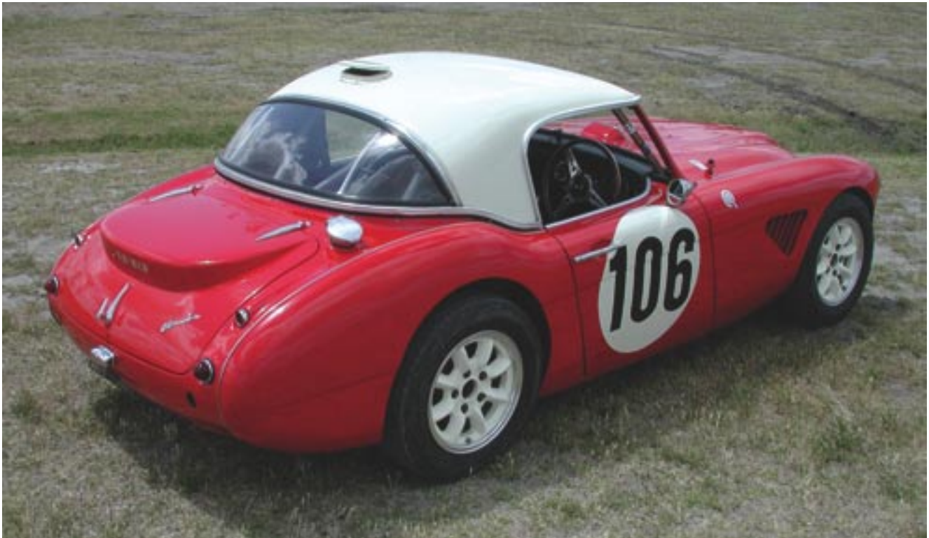
This rear view shows off the “Works” trunk lid that has a bustle for a second spare tire (remember, these were Rally cars). “Works” vented hardtop has a rear-facing vent to improve flow-through ventilation.
