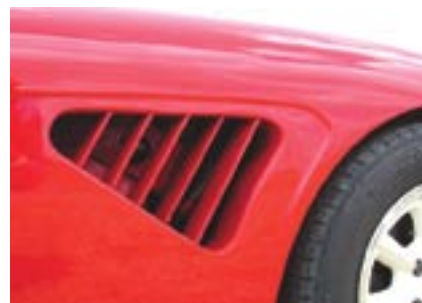
One of the very distinctive characteristics of "Works Rally" Healeys is the unique side vents. Inside fender panels are also lightweight aluminum.
