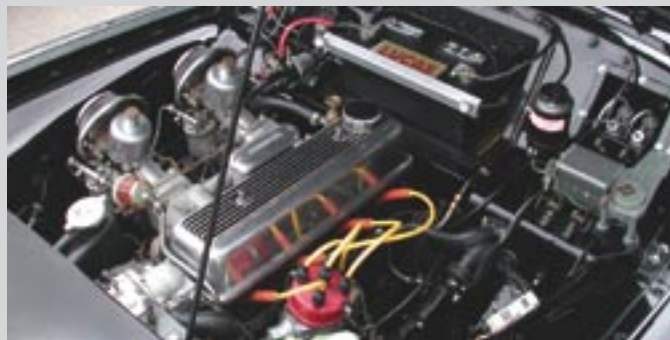
The engine has about 175,000 miles on it. Aftermarket goodies include K&N air filters, a Mallory distributor, and aftermarket plug wires.
