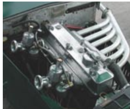
The inline-six-cylinder SOHC MG powerplant now displaces 1430cc and produces 75hp by way of a hotter camshaft and larger SU carbs. Beautiful exhaust is believed to be a genuine NE racecar piece.
