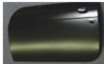
Prep new body panels by sanding their protective coating and using a self-etching primer.
