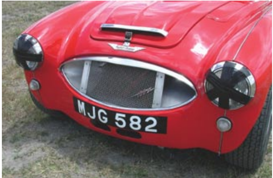
MJG 582 Rally designation was bestowed on #106 by Geoff Healey. “Works” grille provides max airflow and radiator protection. Taped headlights reflect on a bygone era of sportscar racing.
