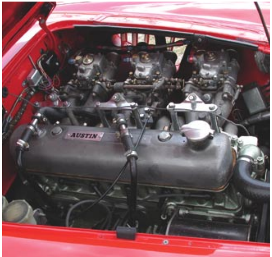
Austin-Healey inline six-cylinder engines are known torque producers. The race version has the best of everything: Nitrited crankshaft, Carillo rods, 11.5:1 J&E forged pistons, Isky cam, “Works” aluminum cylinder head, magnesium intake manifolds and valve cover and a set of “Works” triple 45 D.C.O.E. Weber carbs. Other details include a Denis Welch competition flywheel and a six-branch competition exhaust system that must be heard to be appreciated.
