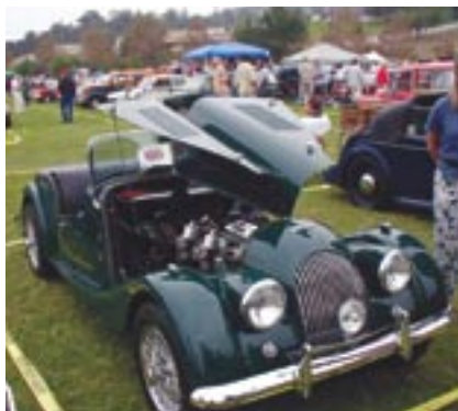
Opening up the cowls at speeds above 40 mph induces negative lift in this Morgan.
