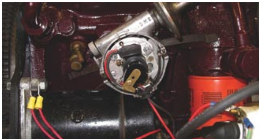
Close-up of the OE generator in relation to the distributor arm.
