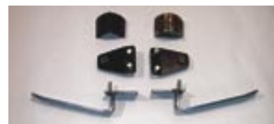
The upcoming Moss conversion kit will include all the hardware necessary to convert rubber bumpers to chrome.
