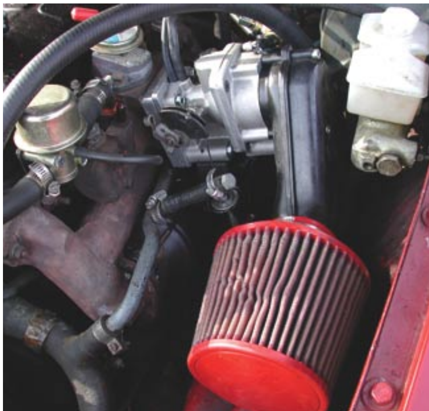
This close-up of the Moss throttle body bolted onto a stock MGB intake shows how clean the installation is. The throttle body has an OE-style bellcrank for the throttle linkage. Air cleaner is from a VW Golf with a K&N clamp-on filter.
