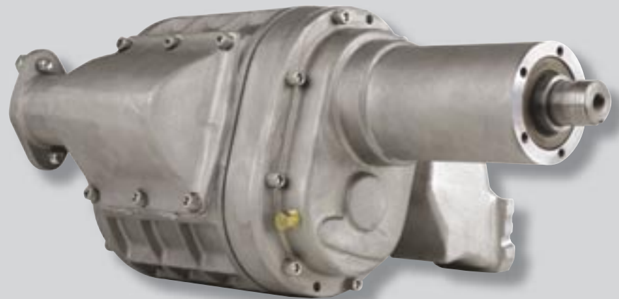
Moss Motors designed its T-Series supercharger case to look like a period Marshall unit. However, inside the housing is a modern-tech Eaton dual-rotor system.
