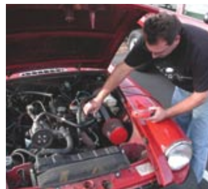
EFI Project Manager Mark Luis checks air-to-fuel ratio parameters. This EFI-equipped MGB drives like no other MGB you've ever driven!
