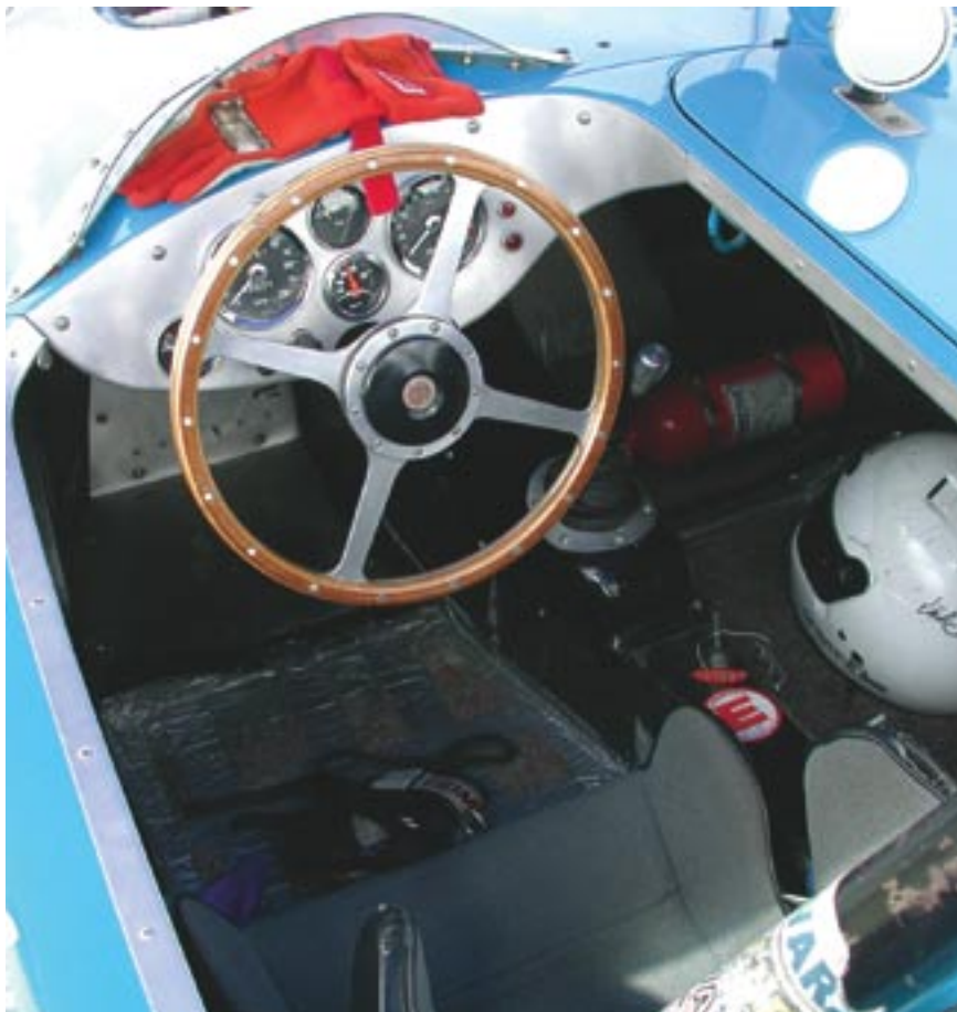
The hand-formed curved-alloy dash holds MGB gauges. A Mota-Lita wood wheel guides the 1,750-pound racer around the course.
