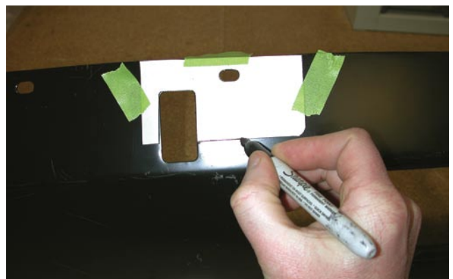
9. The new valance must be notched for the bumper mounting pads with a die grinder or tin snips. Mark it using the instruction's templates.
