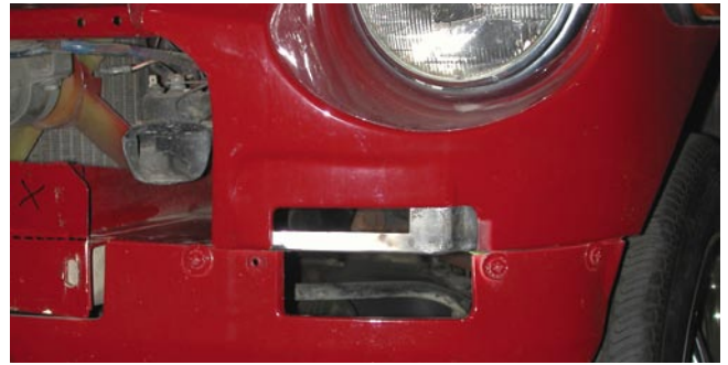
6. Fit and weld the kit's turn-signal filler pieces onto the car.
