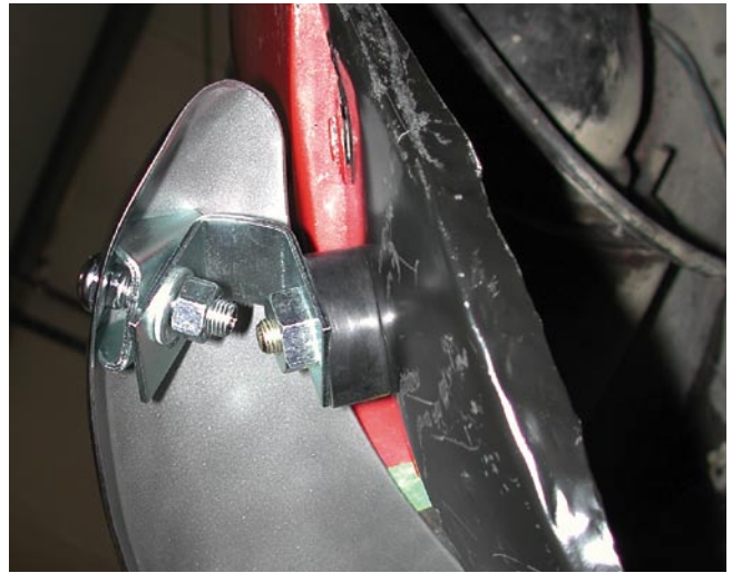
14. Install the kit's corner brackets between the bumper and valance; mark and drill holes. Then the overrides can be attached to the bumper.
