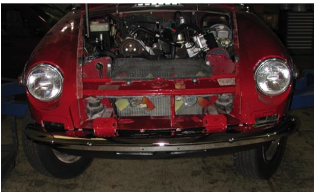
13. Install the bumper on the brackets, adjusting it for proper alignment with the body per the instructions, using the factory shims if necessary.
