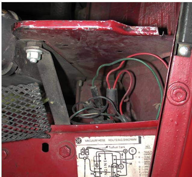
2. Disconnect and label the front blinker/running light wires near the radiator.
