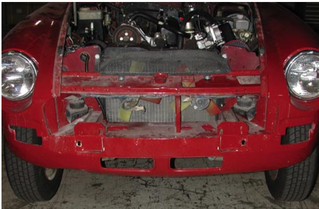
5. Remove the lower mounting nuts, then the uppers. Note any shims between the bumper and car. The bumper removes by pulling it forward; an assistant is helpful here. Guide the wires as the bumper is removed.
