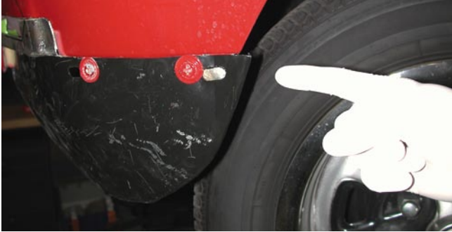
11. Bend and trim the valance's flanges as necessary to align with the fenders. This requires removing the valance.
