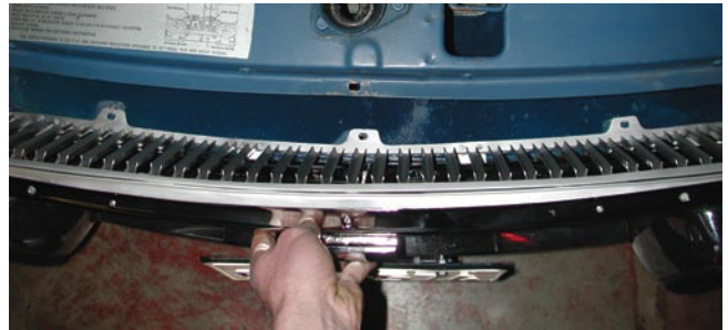
15. Narrow the grille and shape the hood if necessary to fit the new bumper. Set the grille in place and fasten through the bottom holes.
