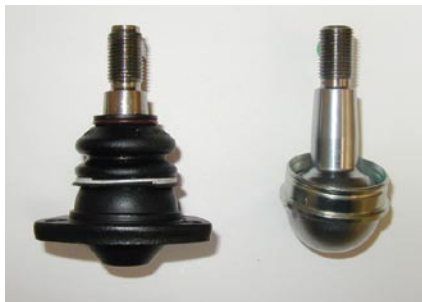
Later XJ6 balljoint (left) compared to earlier socket-style joint.
