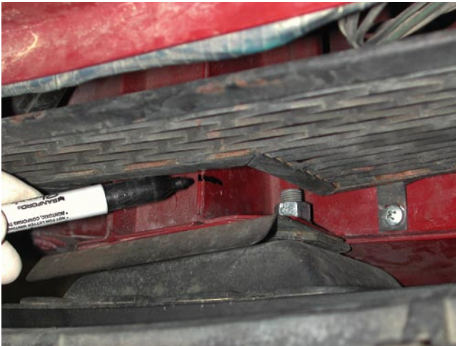
4. Mark the grille's position on the framersails, then remove the grille to access the main bumper mounting bolts.
