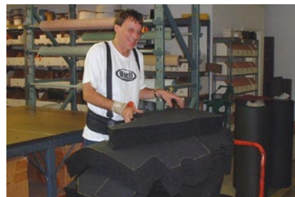
4. Michael shows how carpet pieces are cut and moved in batches of nine. In the background, note how materials are on rollers over the cutting table to maximize speed and minimize lifting.
