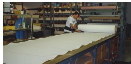
9. Once the pattern is marked on the foam, Michael cuts it out with electric shears. Tools like this allow speed and accuracy compared to original manufacturing processes.
