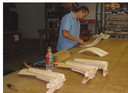
10. These Big Healey rear quarter panels are one of the more intricate components made in the Moss upholstery shop. Here, Sergio applies foam to formed waterboard. The piece will be covered in vinyl later.
