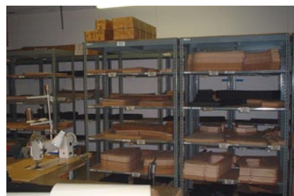
6. Interior panels begin as precision die-cut blanks of wood veneer or black waterboard.
