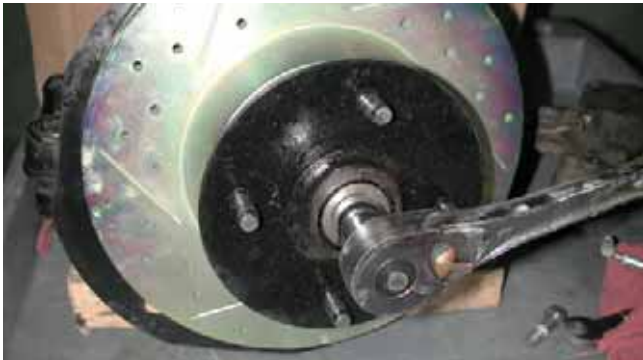
14. Torque the spindle nut to factory spec, then install a cotter pin if the original setup used a castle nut. Pack the dust cap with grease and tap it into place.
