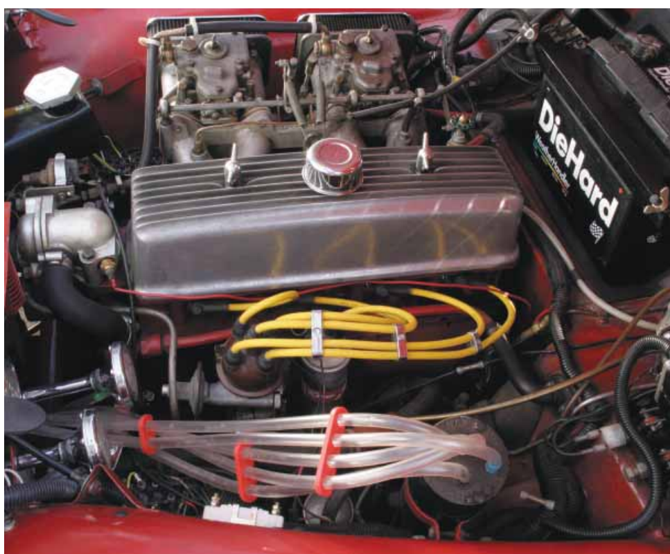
Dual Webers and a chromed header help hot-rod the 2.2L engine. Air lines for the 5-trumpet horn are also visible.
