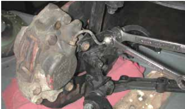
2. Loosen the fitting at the brakeline retaining bracket.
