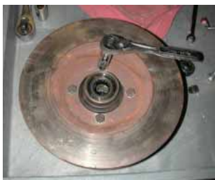
5. Secure the lugs in a vice if necessary, then unbolt the hub from the rotor. Save the lockwashers.
