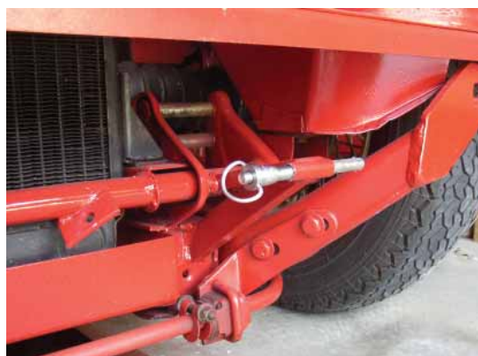
Pull-pins are used to secure the clamshell apron conversion.
