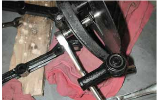
8. Slip the backing plate off the spindle, rotate it to clear the caliper-to-spindle mounting bracket, then remove the plate.
