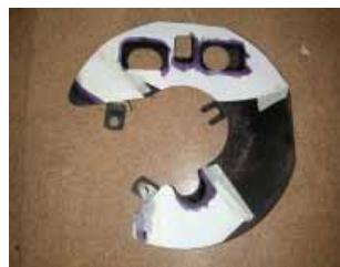
9. Clean the backing plate, then use the kit's template and mark where the plate will need to be cut.
