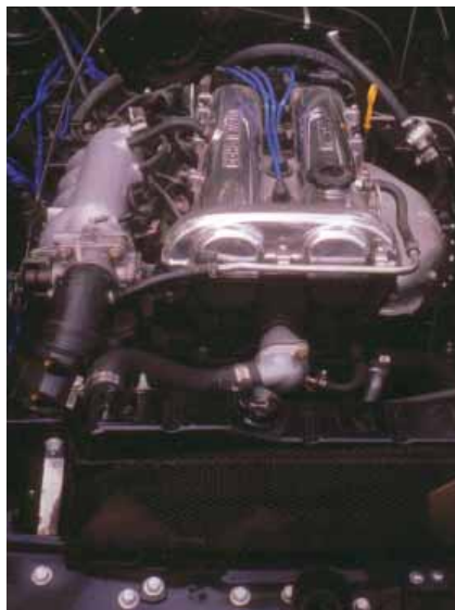
Twin-Cams were popular. This MGB-GT features a swapped-in 1.8L Miata engine.
