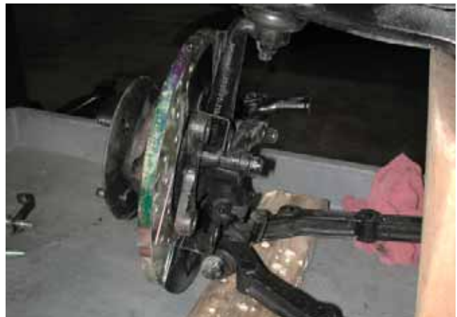
11. Test-fit the modified backing plate with the spindle, bearing, hub/rotor assembly, and caliper. Re-trim the backing plate if necessary to create more clearance, particularly in the caliper area.
