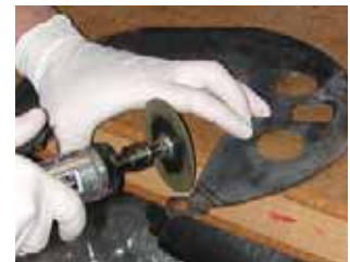
10. Use a cut-off wheel, nibbler, and/or die-grinder to trim the backing plate. File any sharp edges smooth.
