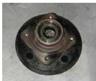
6. This is an opportune time to repack the bearings or replace them and their felt seals. Moss Motors stocks the necessary replacement parts.
