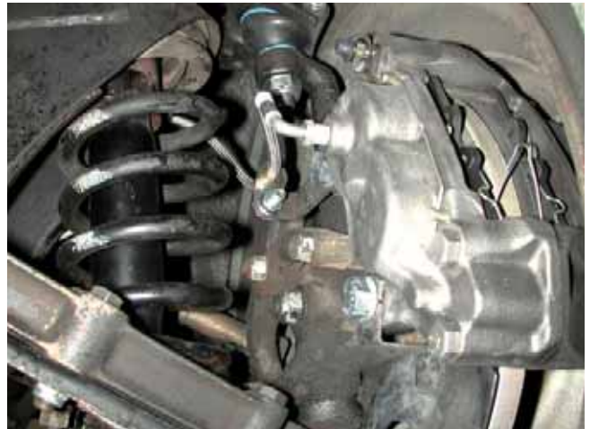
17. Use line wrenches to tighten the hose. Then spin the rotor to verify clearance between it and the pads' anti-squeak spring.
