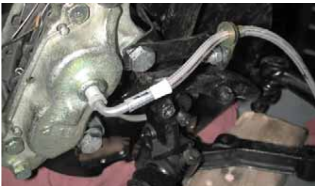
15. Install one of the kit's braided brakelines: Hand-thread the end with a 90-degree bend into the caliper.
