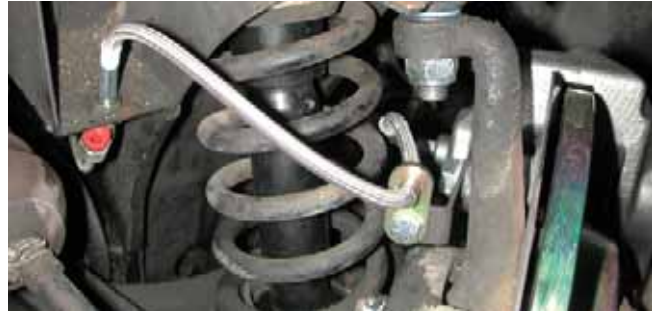
16. Route the hose between or over the coil to clear the spring during suspension movement. Move the line's crimp to its line locator and use the kit's hardware to secure to the factory retaining bracket.
