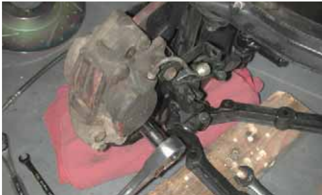
3. Remove the lower caliper bolt first, then hold the caliper while loosening the upper bolt. Pull the caliper from the splash-shield and spindle mounts, then remove it from the rotor. Save all brackets and spring washers.
