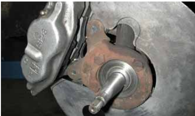
13. Check again for interference between the caliper and backing plate.
