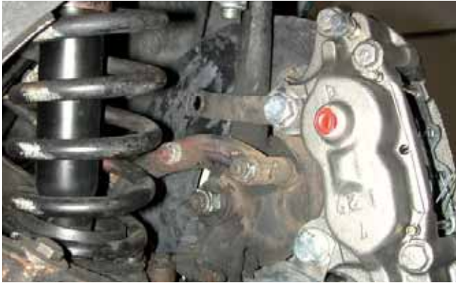
12. The kit's calipers are marked Left and Right. Mount the caliper with the bleeder screw facing up. Then mount the L-shaped brakeline bracket horizontally.
