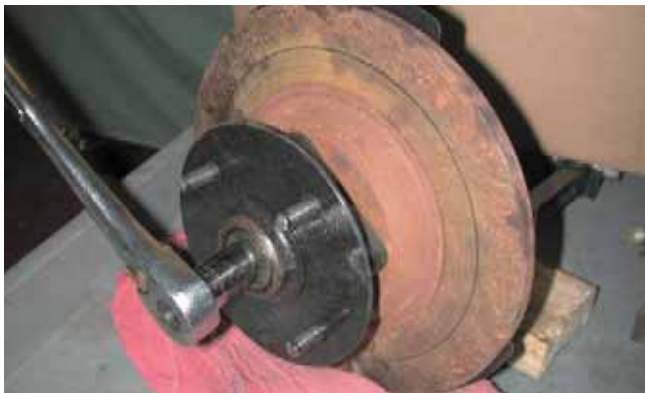
4. Wiggle off the hub dust cap with vise grips. Then remove the cotter pin (if equipped) and the spindle nut. Remove the rotor/hub, saving the bearing and washer.
