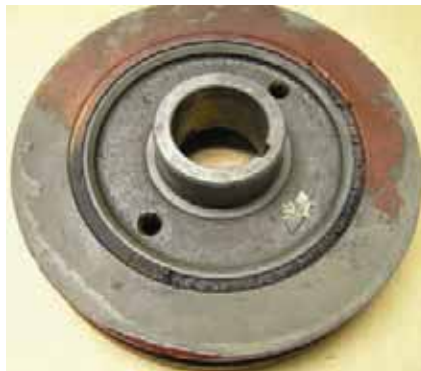
4. The inside of the damper and the oil seal surface were both clean and smooth. There was no apparent damage to the rubber damper, and Evapo-Rust won't eat away paint or plating.
