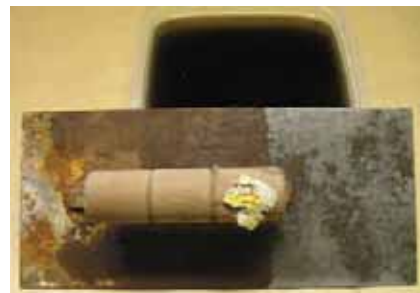
8. This is the tool after sitting overnight in Evapo-Rust, ambient temperature around 45 degrees. Even so, the results were impressive.
