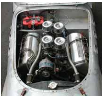
The Allard has a very impressive Arduin-converted Flathead Ford engine. It features period-correct carbs on a log style manifold. This engine is music to any racer's ears.
