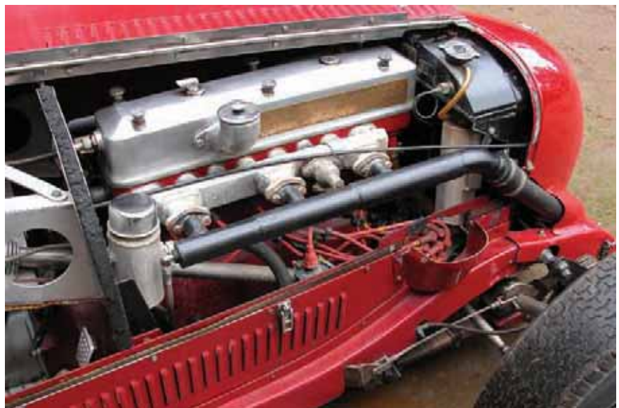
The MG 1100cc inline six-cylinder gets fed boost from a front-mounted supercharger. An intake tube travels back to the engine, pressurizing the three-port intake manifold.
