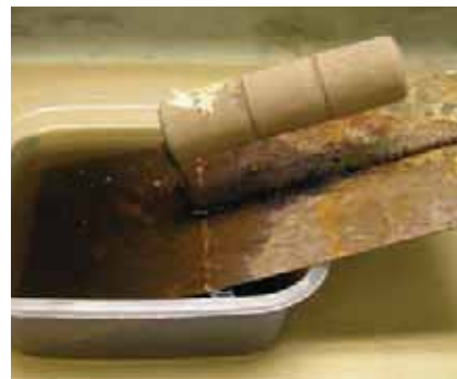
7. Next up was the concrete finishing tool, which seemed like a good example of how Evapo-Rust works on steel.
