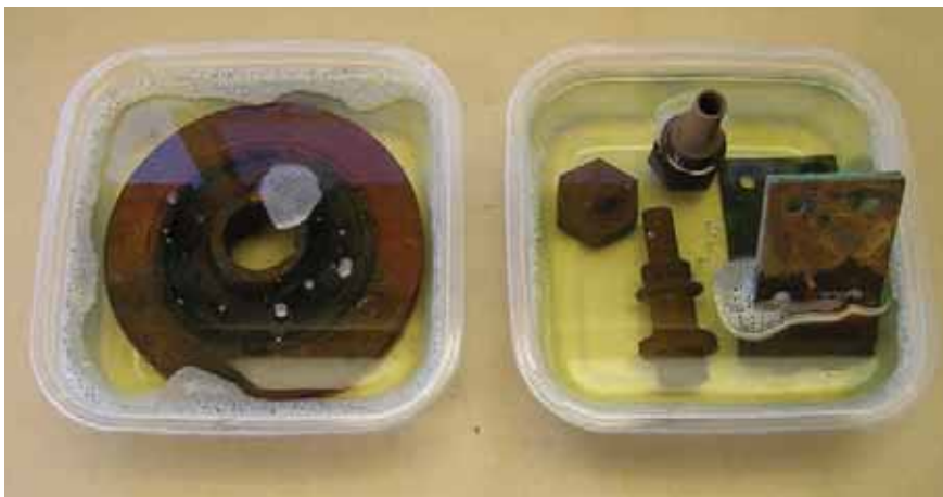
2. Pour Evapo-Rust into a suitably sized plastic container, possibly one purchased by the wife at a party. Completely submerging the parts produces the best results, but we dangled a few bits out for before-and-after comparisons.
