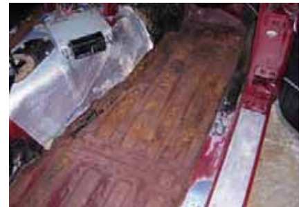
5. Before cutting out the old pans, measure and re-measure the locations of the seat nuts and line clamp studs. Transfer these dimensions to the new pans.
