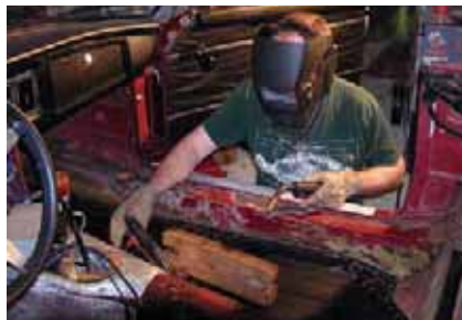
14. To assure good welds, we used two hammers (one under the panel as a back-up) to flatten the drilled holes.
