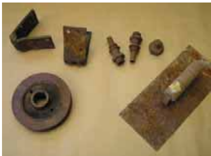
1. The test subjects: an MGB harmonic damper that sat in mud, a pair of MGA door hinges in pre-resto condition, a pair of oil cooler fittings, and a crank bolt that was degreased, then sat for 10 years. (The concrete tool sat out in the rain, just to prove there is life after British cars.)
