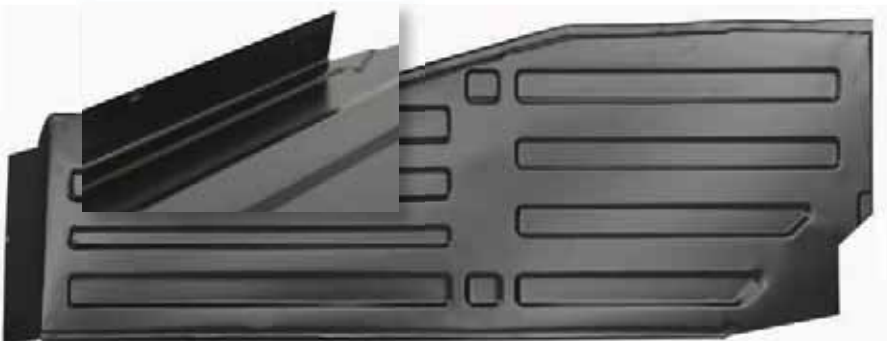
3. Instead of welded-on nuts and studs, replica pans (P/N 458-950, 458-955) have an extra 1" vertical lip of sheetmetal all around.
