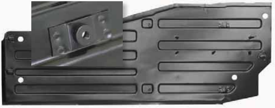
2. Both OE and reproduction floor pans are available for the MGB from Moss. The OEM replacement pans (P/N 458-885, 458-875)—one per side—have the nuts for the seats and the studs for the brake and fuel-line clamps already welded in place.
