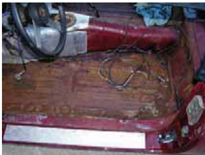
4. Replica pans were chosen here because of their extra "meat" for the rusted-out transmission-tunnel sheetmetal.
