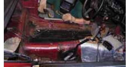
16. Spot-weld the new panel in place. (Always have a fire extinguisher on hand—better to have it and not need it than the other way around.)
