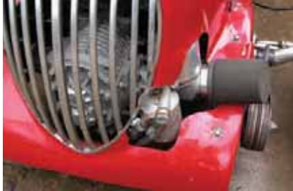
A vintage Volume-Ex supercharger is driven off of the front of the crankshaft and draws fuel through a large Solex carb that extends through the grille shell.
