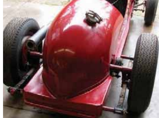
The rear of the L-Type is pretty basic with semi-elliptical leaf springs, N-Type axle and friction shocks. The modern Supertrap exhaust is the only way to dampen the piercing exhaust note.
