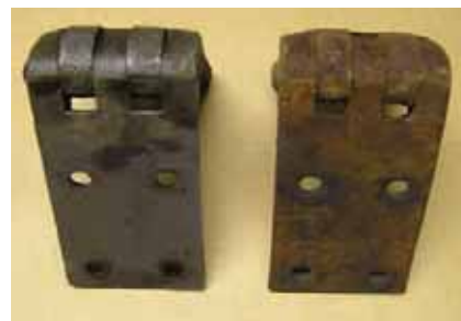
6. This shot of the MGA hinges shows the striking difference after the bath. The right-hand hinge didn't taste Evapo-Rust.
