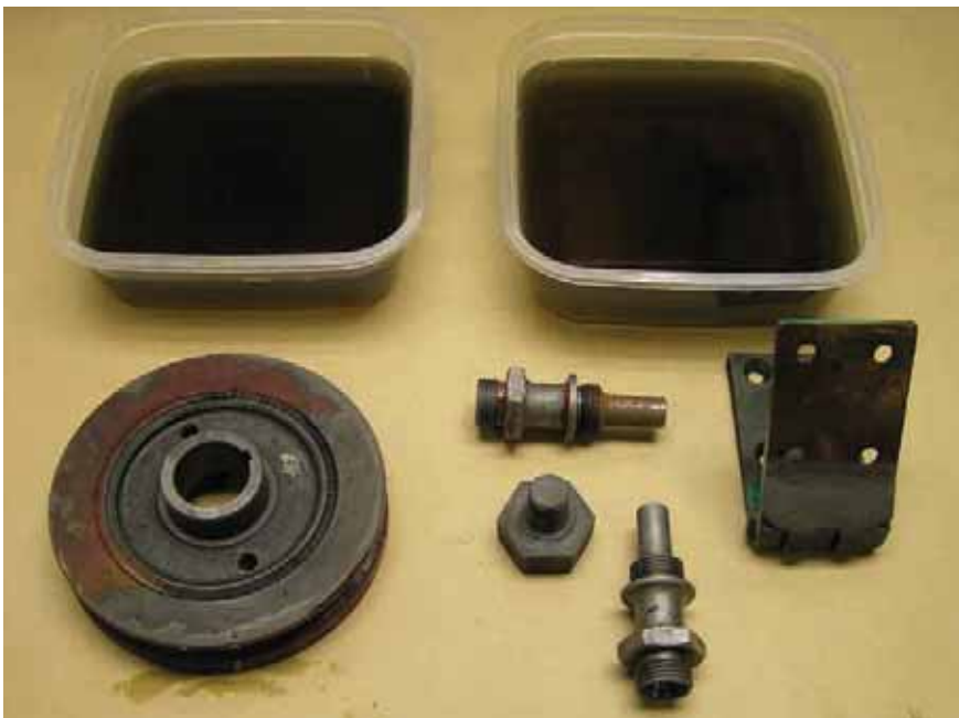
3. The next day, this is what the parts looked like after rinsing with tap water and drying. Evapo-Rust turns from clear to black as it works, indicating how much rust was removed. The same bath can be reused until the product won't work anymore.
