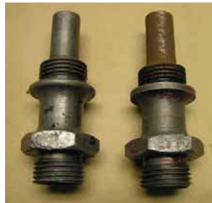
5. This close-up shows the difference between the oil fittings: The one on the right was only partially submerged. Inside the fittings, the red oxide has been completely removed.
