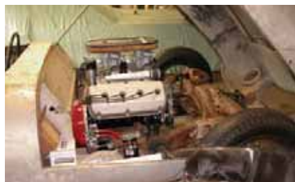
A pristine 354cid Chrysler Hemi will power the Challenger. It is riding in a '49 Ford chassis with an independent rear suspension.
