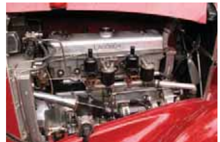
Dual carbureted, the Lagonda inline six cylinder is beautifully detailed. George claims it has a lot of torque and is an excellent high-speed cruiser.
