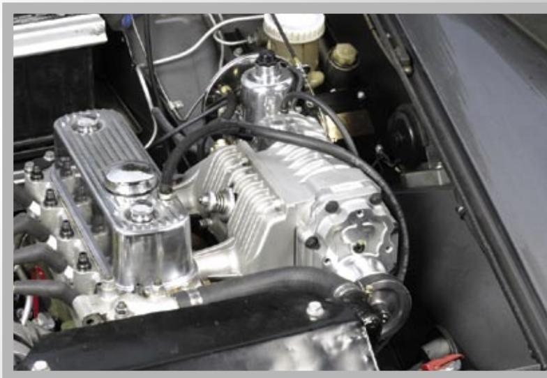
Main components are an Eaton M45 (45 cubic-inch displacement) supercharger and a Moss-designed manifold. The system was designed to look like a factory option instead of an aftermarket upgrade.
