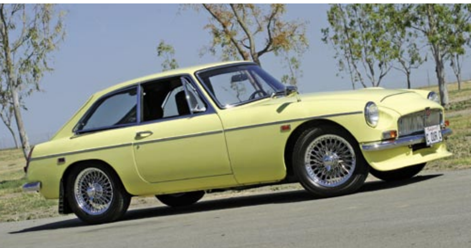
Bob and Sandie added the air dam to help direct air to the engine bay for better cooling. Plus, they like the way it looks.
