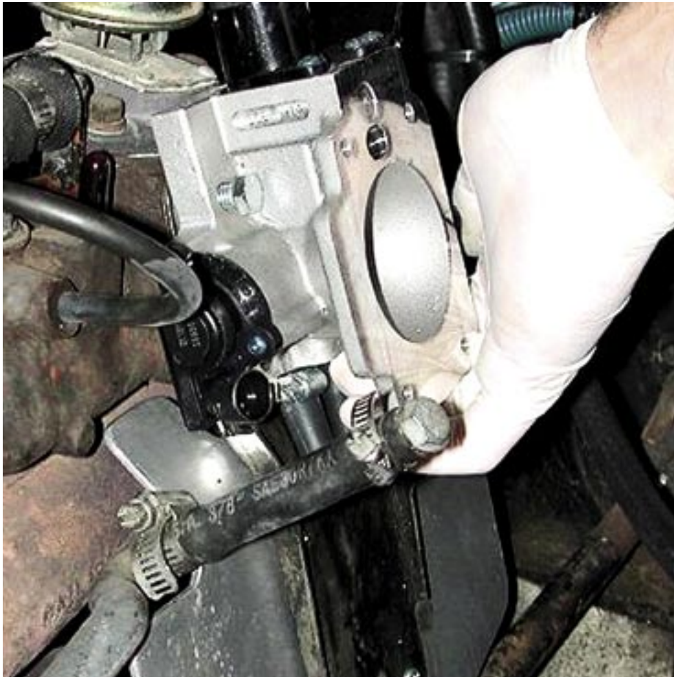
10) Offer up the throttle body and heat shield assembly to the intake manifold. Tighten the four retaining bolts.
