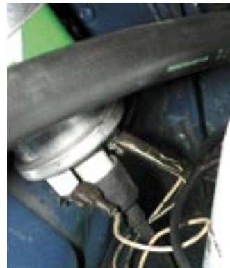
14) The ECU needs to have a feed from the tachometer to monitor engine speed, so one of the wires in the harness is attached to the distributor and another is placed on the negative side of the coil. A third tachometer lead comes out of the box to provide a signal for the tach.
