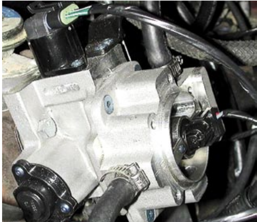
12) Next, we have to connect the harness to the throttle body. The wire loom has plugs for the idle air control motor, fuel injector, and throttle position sensor. All three connectors are unique, and there is no way to make a mistake plugging them in.
