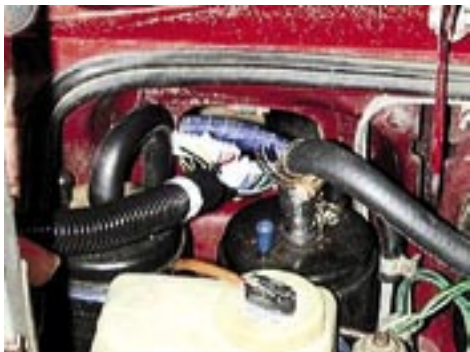
11) The brain of the EFI system is an electronic control unit, or ECU. The box is housed inside the cockpit under the dash, and a pre-fab wiring harness has to be routed through the firewall. Remove the right hand side under-dash panel and find the rubber grommet in the firewall and remove it. Cut a one-inch hole in the grommet and reinstall it; this is where the wiring harness will pass through.
