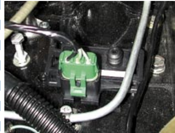
13) Part of what makes EFI systems so efficient is the MAP sensor, which monitors the difference between the pressure inside the intake manifold and atmospheric pressure outside the manifold. The ECU processes the info to determine engine load, and adjusts fuel flow accordingly. Plug the sensor into the harness, and mount it in the engine compartment.
