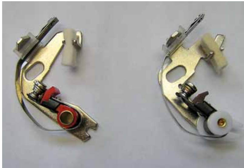
The DSB108 as fitted to the Lucas 41427 and 1975 Federal applications is on the left. The DSB191 self wiping point set is on the right, the points are wiped across each other as the white lever to the bottom of the point set is moved.
