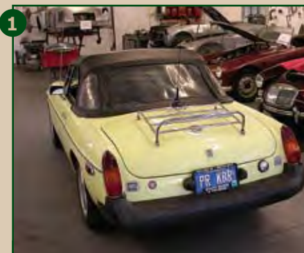
1 This MGB's top was about 15 years old. The back window had yellowed and many of the snaps were torn out. The time had come for a new top.
