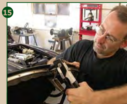
15 Then we riveted the header seal channel into place.
