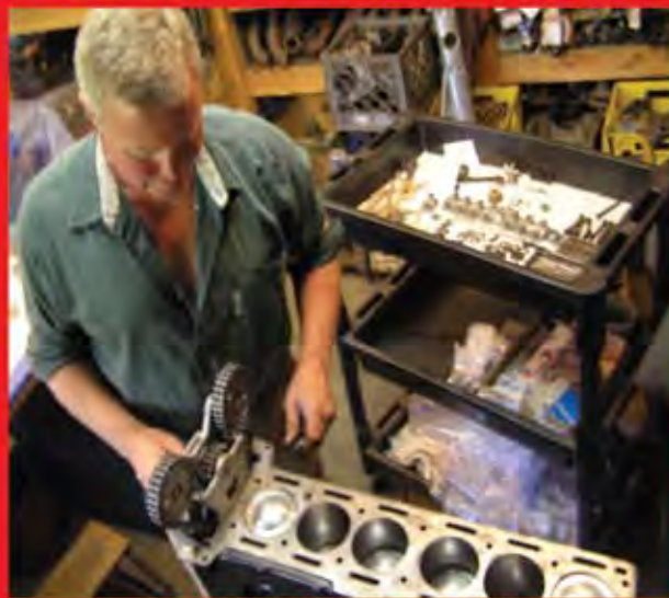
David Clark assembles a 3.8 litre E-type engine
