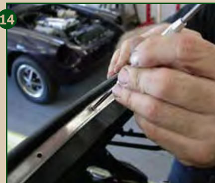
14 We planned to reattach the header seal channel with rivets, so we used a dentist tool to poke holes in the top material.
