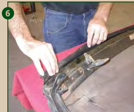
6 We pulled and unglued the old top from the header rail.
