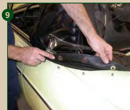
9 We repaired several worn-out snap studs, and then snapped the new top into place at the back.
