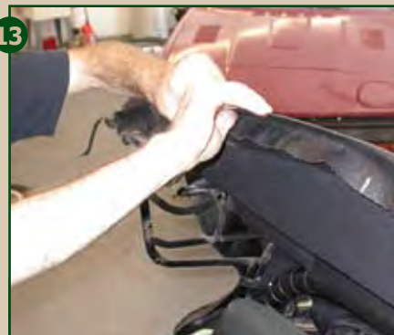
13 Once we were satisfied with the fit of the top, we folded the excess material underneath the header seal channel area.
