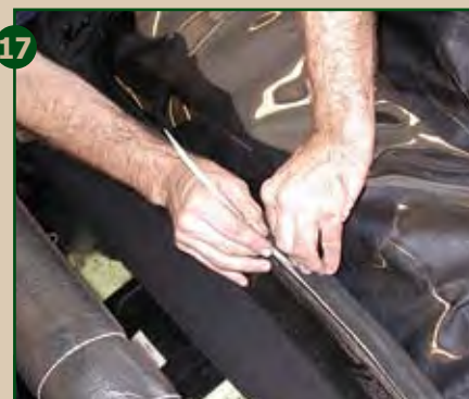
17 We installed the header seal using a special plastic tool used by windshield installers. If we didn't have the tool, a paint stick or even a screwdriver would have worked fine.
