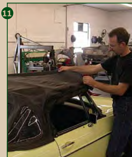
11 We pulled the top tight to the windshield and header rail.
