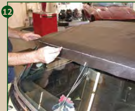
12 We marked the front edge of the top, then put some witness marks at the center and sides. As we made adjustments to the top for fit, we re-marked these lines.
