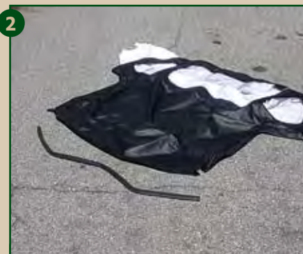
2 Before we started the job, we laid the new top and header seal in the sun to let the fabric become warmer and therefore more pliable.
