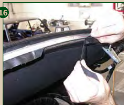
16 Using a razor blade, we trimmed away the excess material.
