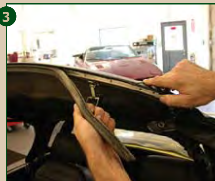
3 We started removing the top by unlatching the header rail and pulling away the header seal, revealing the aluminum seal channel and attachment rivets below.
