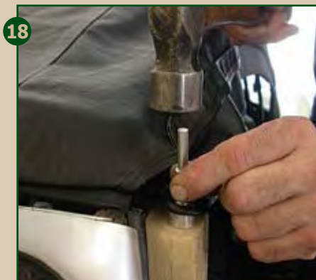
15 Then we riveted the header seal channel into place.
