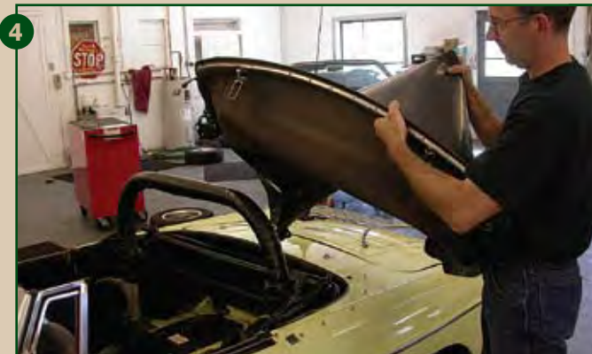
4 We completely removed the header rail from the car by undoing three screws on each side.
