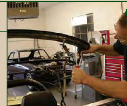
7 We reattached the header rail to the top bows.
