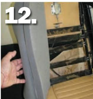
**▲** Next up is the seat back. First, recover the area behind the headrest. If you have a 1969 TR6, reinstall the headrest latch. From there, follow roughly the same procedure as for the seat bottom, gluing on the seat back cushion and then attaching the seat cover with clips on the back of the seat.
