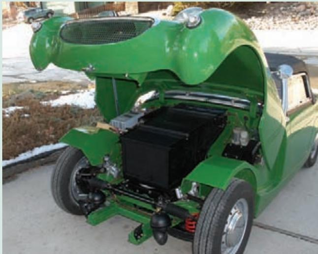
**Top:** The Bugeye nose hinges up for full engine access. **Below Left:** The nine lead acid batteries charge in two to eight hours. **Below Right:** The weight from the batteries was offset by upgrading suspension with heavy-duty front and rear springs. **Bottom:** Little Go Green generates lots of interest at car events, a classic car with eco ethics.
