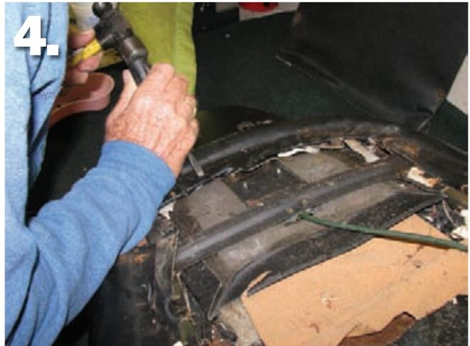
▲ Flip the seat over, and knock off the clips that hold the seat bottom and back covers in place.
