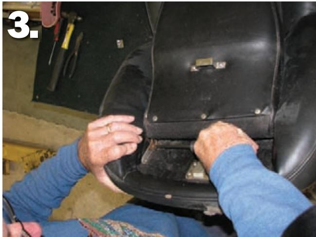
▲ Start by taking your old seat apart. The back comes off first and then (on a '69 TR6) the headrest comes off with four screws.
