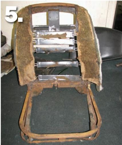
**▲** Remove the seat cushion material, straps and the cardboard piece behind the headrest. Once down to a bare frame, clean it with a bead blast cabinet; a wire brush and elbow grease also does the job. Then give the frame a fresh coat of paint.
