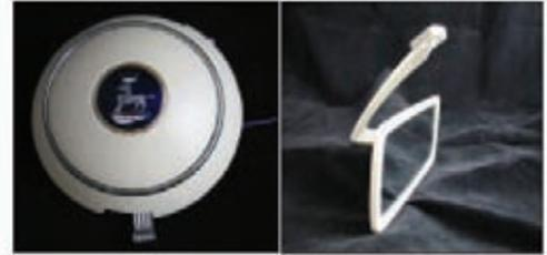
Remanufacturing examples of horn button (left) for Sunbeam Talbot, and rear view mirror (right) for Ford Consul Cortina.
