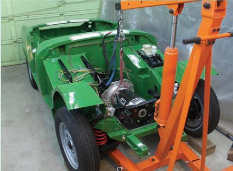
**Left:** This '62 Sprite waited a long time for restoration, surviving a wreck, a fire and 30 years of storage before getting a chance to illustrate how green a British car can go. **Below:** The electric car gets 50 miles on a battery charge with a top speed of 70 mph and an amortized cost of 5 to 7 cents-per-mile for operation.
