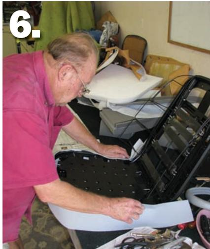
**▲** Begin reassembly by reinstalling the bottom seat cushion diaphragm, followed by the seat back straps and the foam skirt around the seat bottom.
