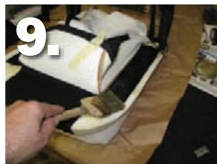
**◀** Tape the edges of the seat cover out of the way and glue the attachment cloth pieces to the seat cushion. Make sure the seat cover is centered correctly. Then put more glue over the attachment pieces to add more foam around the seat cushion. Remember to always glue both sides and wait a few minutes for the glue to dry.
