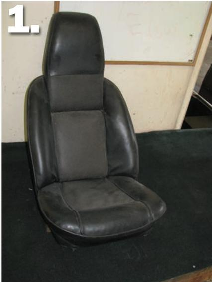
◀ You can tell the foam underneath our TR6 seat has disintegrated since the seat cover no longer fits on the seat correctly. While this seat might not look that bad, the comfort factor in saggy, old seats doesn't compare to restored seats.
