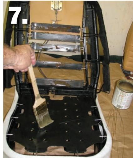
**▲** Brush glue onto the diaphragm to hold the bottom cushion in place. Use brush-on contact cement available at hardware, upholstery supply and building supply stores. Don't use spray glue; we found it doesn't hold up due to the heat and moisture inside a car.
