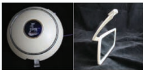
Remanufacturing examples of horn button (left) for Sunbeam Talbot, and rear view mirror (right) for Ford Consul Cortina.
