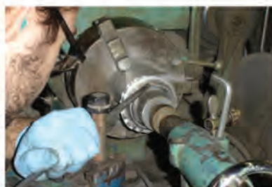
Craftsman using spinning technique to produce bezel for Lucas lamp assembly.
