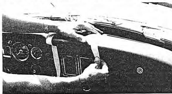
3) Apply a bead of adhesive (provided with the panel) to the underside of the repair panel. Position the panel on top of your rotted dash, using tape to hold down the edges as necessary. Heavy objects (phone books etc.) should be placed on the pad to ensure a tight fit. Let 'cure' for 24 hours.
