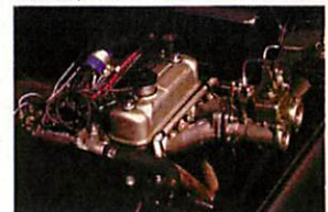
Left: The flaming Midget, as built by Original Duplicates in Fresno, CA. Above: Cheshire grin and wider tires. The MG medallion is mirror imaged so folks can tell what's behind them. Right: Bugeye intake manifold leaves no room for an air cleaner. Caution - birds and small children stand clear of the Weber.
