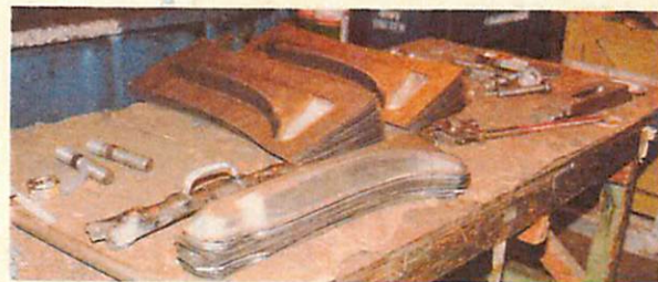
Two steps in the reproduction of rocker panels. In the rear, freshly stamped panels, in the foreground, the same panels are trimmed and ready to be shipped.
