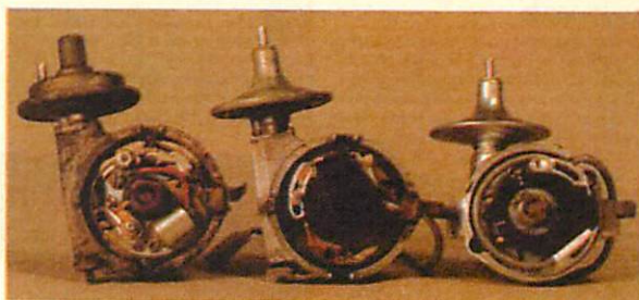
Left to right: Early "point-style" MGB distributor; same unit with XR-700 installed; late "electronic" MGB distributor with XR-700.
