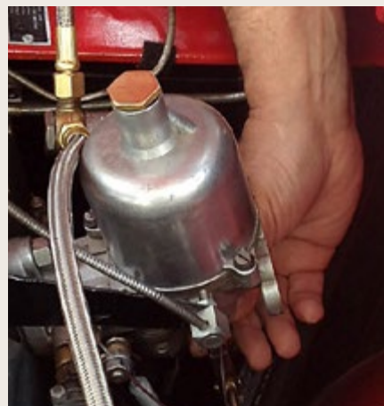
Fuel mixture nut (bottom of carb) is adjusted by hand, one flat at a time... up=leans, down=enriches.
