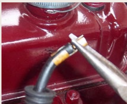
Brass contacts on plug wires are squeezed for a tight fit.
