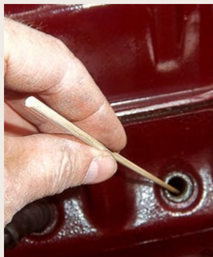
Rising skewer confirms top of piston travel.
