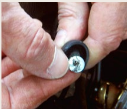
A new washer was fitted to the coil end of the distributor to coil wire.
